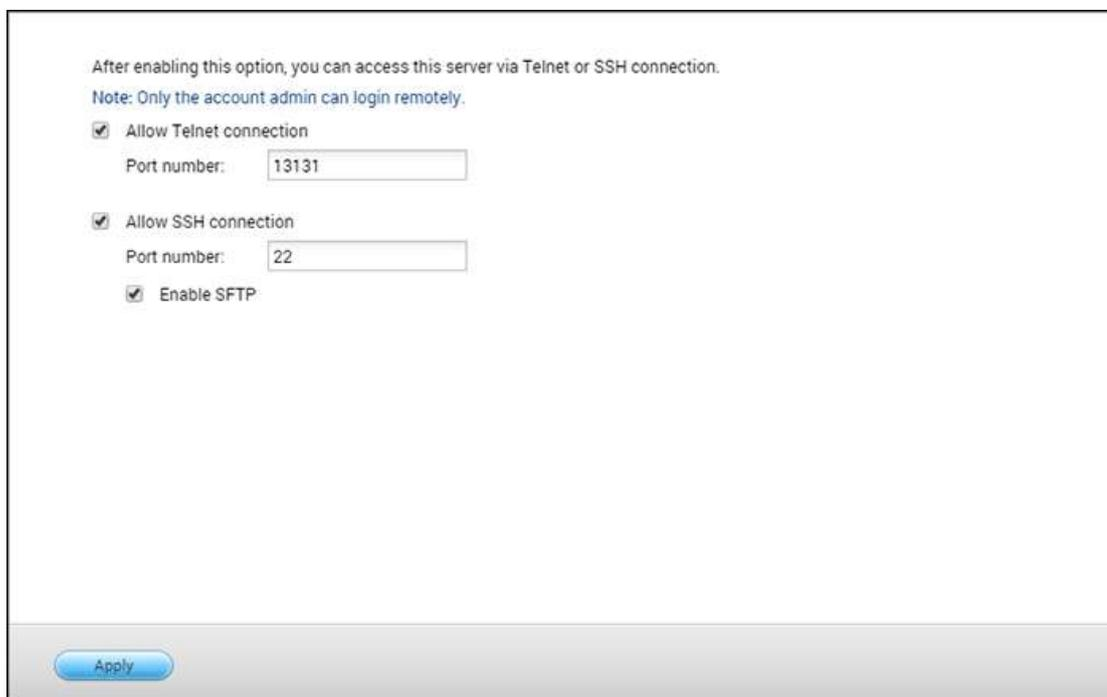
After enabling this option, you can access this server via Telnet or SSH connection.
