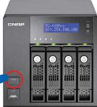
After installing the hard drive(s), connect the power cord to the NAS. Plug the other end of the power cord to the wall socket and turn on the NAS.
