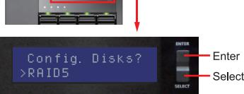
The system detects the number of hard drives installed and prompts you to execute the default configuration. Press "Enter" to confirm.
