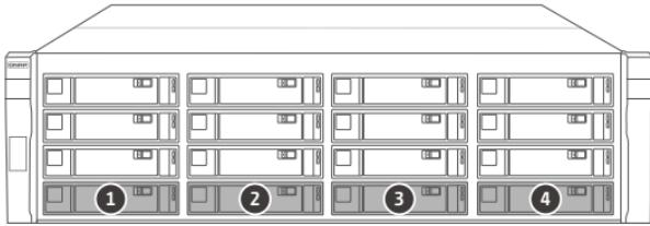
QES uses drive bays 1-4. QNAP recommends using SSD drives for QES - - - - - [en](#)
