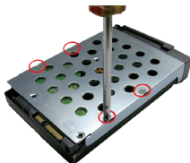
For 3.5-inch HDD (4 screws required)
