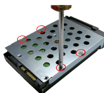
For 3.5-inch HDD (4 screws required)
