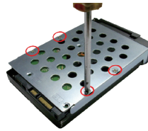
For 3.5-inch HDD (4 screws required)
