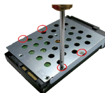
For 3.5-inch HDD (4 screws required)
