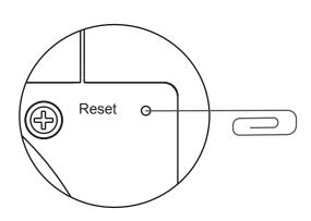
To revert to the default password, use a pin to press the Reset button for three seconds or until you hear a short beep--en
