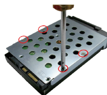
For 3.5-inch HDD (4 screws required)
