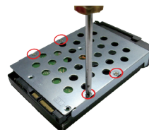
For 3.5-inch HDD (4 screws required)
