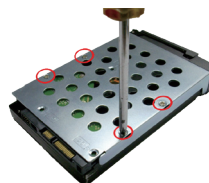
For 3.5-inch HDD (4 screws required)
