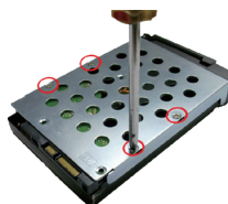
For 3.5-inch HDD (4 screws required)
