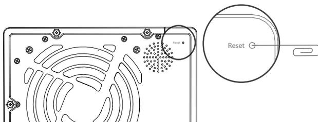
To revert to the default password, use a pin to press the Reset button for three seconds or until you hear a short beep – en
