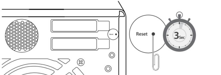
To revert to the default password, use a pin to press the Reset button for three seconds or until you hear a short beep - - en
