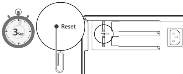
To revert to the default password, use a pin to press the Reset button for three seconds or until you hear a short beep - - en
