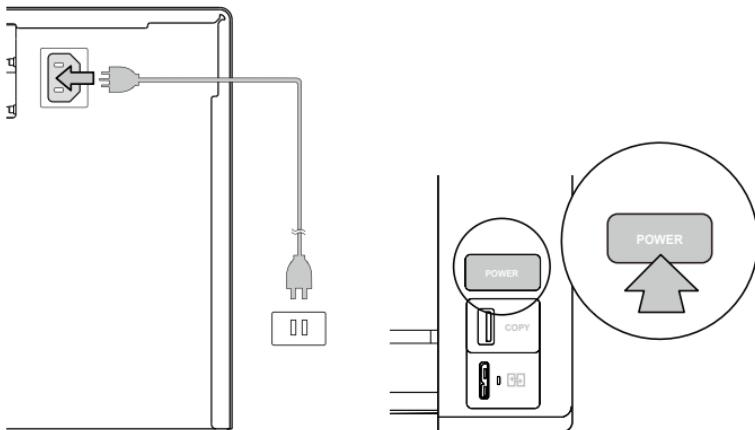
Plug the power cable into the NAS, and into the power outlet - - - - - en
