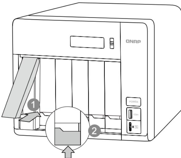
Insert the drive tray into the NAS, and close the latch-
