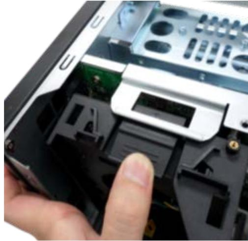
4. Pull the retention clips on each side so that the module can be removed. Remove the installed memory modules.
