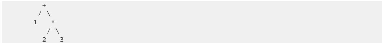
From this AST fragment, you can infer that the multiplication of 2 and 3 happens first (even though `*` occurs textually after the `+`), and the result is added to 1. If the input is instead `(1+2)*3`, then the AST is:
