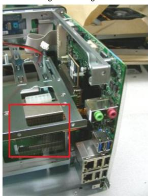
3. Put the back plane into the motherboard and fasten the screws on the highlighted areas.
