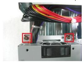
6. Remove the cable tie and disconnect the cable from back plane.
