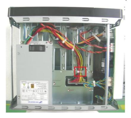
7. Remove the four screws on the motherboard. (When you loosen the top-left screw, it will void the warranty. However, if you correctly followed this guide to upgrading the memory, it will not affect your original warranty\*.)
