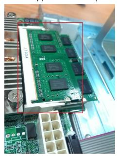
You have finished upgrading the memory. Now, please reverse this process to reassemble the NAS.
