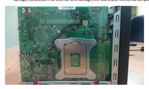
8. Remove the screw on the frame.
