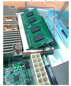
13. Gently press the memory module into the slot until it is seated fully.
