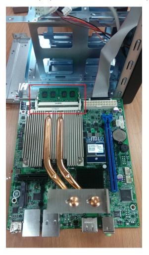
12. Grasp the edge of the memory module. Align the notch on the gold edge of the module with the notch in the memory slot. Slide the memory module to the slot at a 45-degree angle (approximately).
