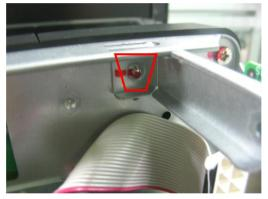
9. Remove the screws from the indicated areas and remove the back plane.
