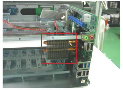
3. Put the back plane into the motherboard and fasten the screws on the highlighted areas.
