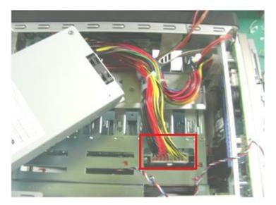
7. Remove the four screws on the motherboard. (When you loosen the top-left screw, it will void the warranty. However, if you correctly followed this guide to upgrading the memory, it will not affect your original warranty\*.)
