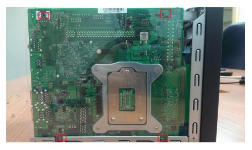
8. Remove the screw on the frame.
