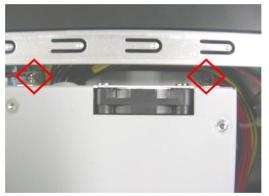
8. Fasten the eleven screws on the rear of the NAS.
