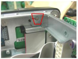
6. Fasten the screws on the motherboard.
