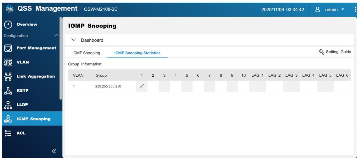
The screenshot shows the QSS Management interface for device QSW-M2108-2C. The main content area is titled "IGMP Snooping" and includes a "Dashboard" section with tabs for "IGMP Snooping" and "IGMP Snooping Statistics". A "Setting Guide" link is also present. Below this, there is a "Group Information:" section with a table:
