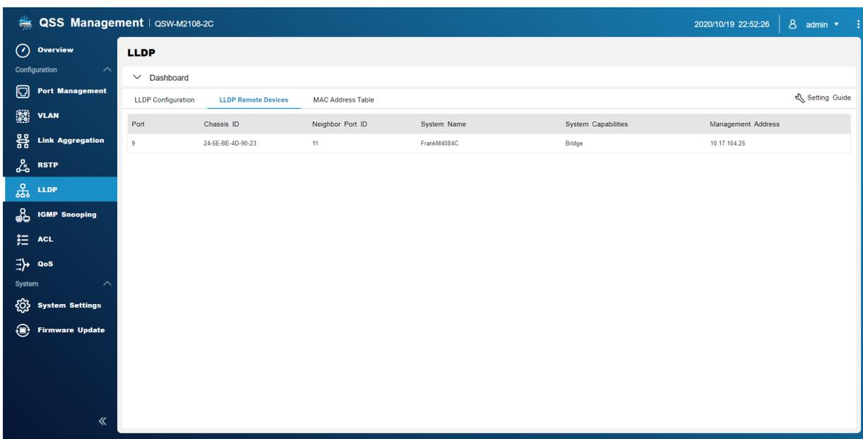
The screenshot shows the QSS Management interface for device QSW-M2108-2C. The left sidebar contains navigation options under 'Configuration' and 'System'. The 'LLDP' option is selected. The main content area shows the 'LLDP Remote Devices' configuration page with a 'Dashboard' tab. Below the dashboard, there are three tabs: 'LLDP Configuration', 'LLDP Remote Devices', and 'MAC Address Table'. The 'LLDP Remote Devices' tab is active, displaying a table with the following data:
