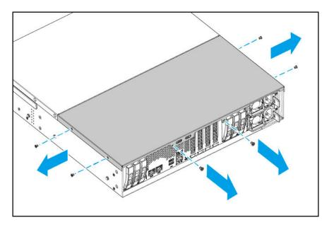
**a.** Remove the screws that secure the rear top cover to the chassis.
