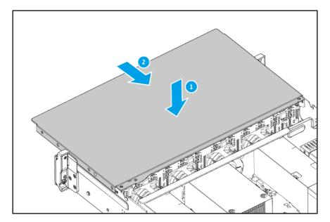
**c.** Attach the screws that secure the front top cover to the chassis.
