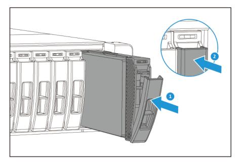
**b.** Push the handle to secure the tray in place.
