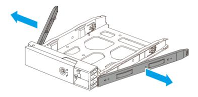
**b.** Place the drive on the tray so that the holes on the sides of the drive are aligned with the holes on the sides of the tray.
