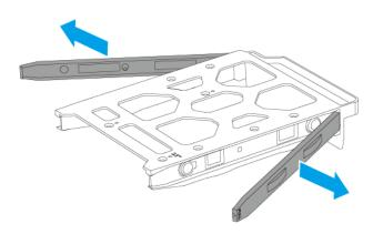
**c.** Place the drive on the tray so that the holes on the bottom of the drive are aligned with the holes on the bottom of the tray.
