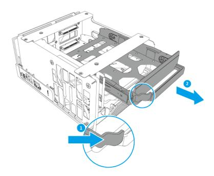
**b.** Remove the fastening panels from the sides of the drive tray.
