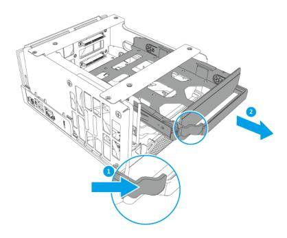
**b.** Remove the right fastening panel from the drive tray.
