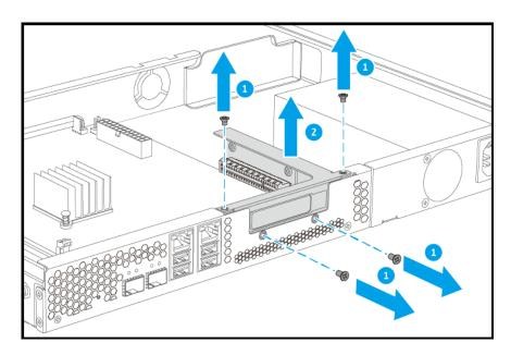
**b.** Remove the bracket from the chassis.
